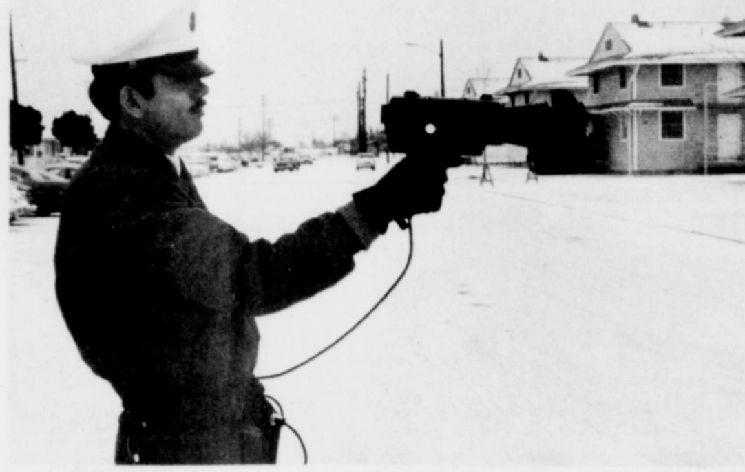
SHEPPARD AFB, TEXAS--CHECKING AUTO SPEEDS--Sergeant John H. Edwards demonstrates the new speedgun, which Sheppard security police will begin using for enforcement Friday. The versatile mobile radar units may be hand held or mounted in cars and have an effective range up to one mile. The exact speed of autos at which it is aimed is provided in a digital readout on the back of the instrument. (OFFICIAL USAF PHOTO)
