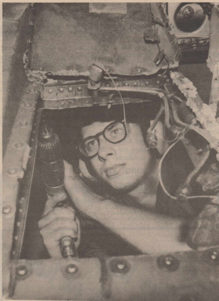
A1C Guy Lensert, assigned to the 64th Field Maintenance Squadron, replaces rivets in a T-38 boattail. He has been assigned to Reese for two years as a Sheet Metal Technician. (USAF Photo)
