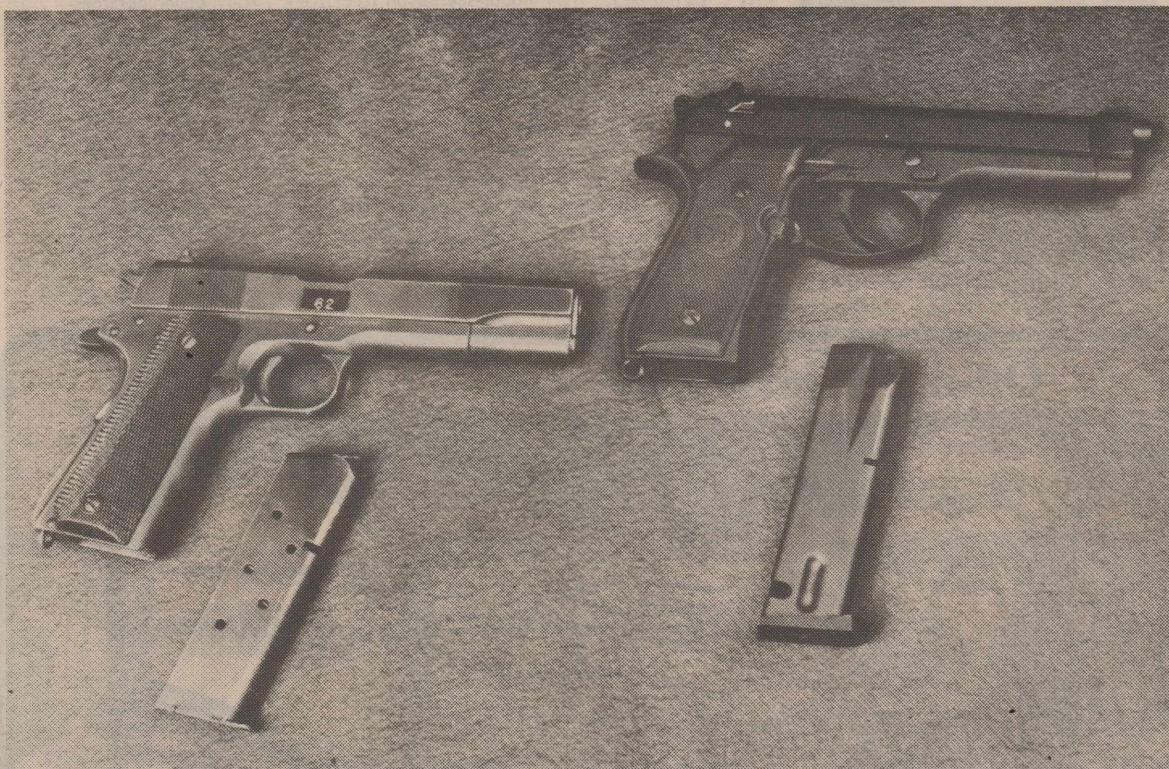
The Colt .45 caliber automatic pistol (left), on active duty since 1911, will retire from military service. The replacement is the 9mm Beretta, which is lighter than its predecessor, holds 15 rounds and fires with greater muzzle velocity.
