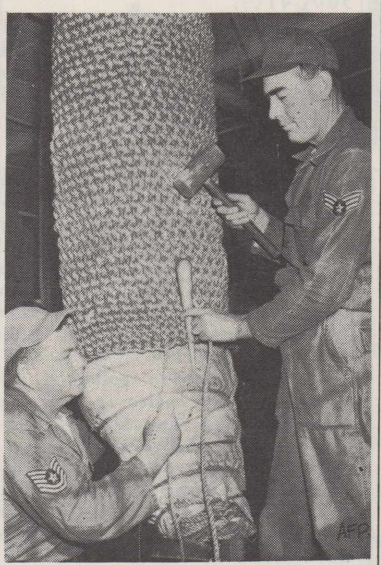
BOAT BUMPER —TSgt. Willard Davis, left, and A1C Arthur Farrell of Eglin AFB are constructing a huge tug boat bumper weighing more than 400 pounds and composed of more than 3,000 knots. When completed, the bumper will be chained to Eglin's 65-foot harbor tug.
