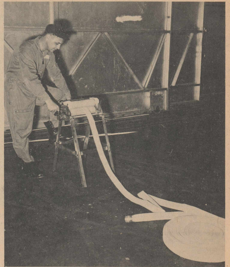
NEW IDEA—A1C Bobbie J. Bunch, Det. 13, Western Air Rescue Service, demonstrates a hose wringer he invented recently and is turning in as an management improvement suggestion. The hand-operated device is made from old washing machine parts and angle iron. The unit uses it to wring out and flatten their firefighting hoses before coiling.
