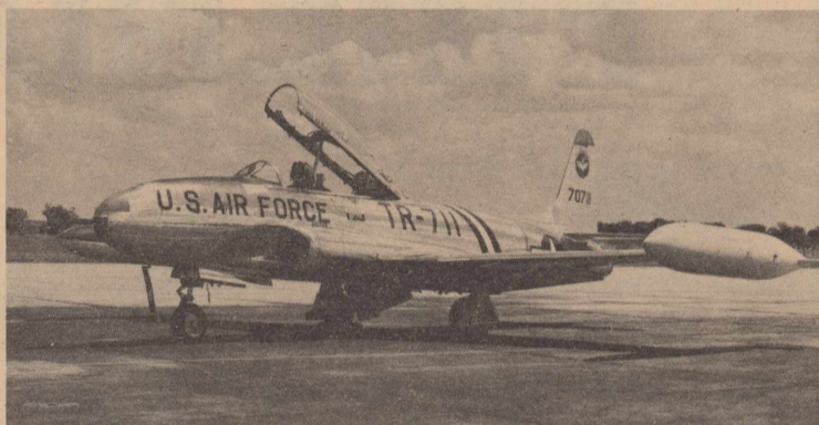
T-BIRD — The first CSAF jet trainer, the T-33 is used by many friendly nations around the world. About nine of ten foreign jet pilots have flown the "T-Bird," including many who trained at Reese before the T-38 was phased out recently.
