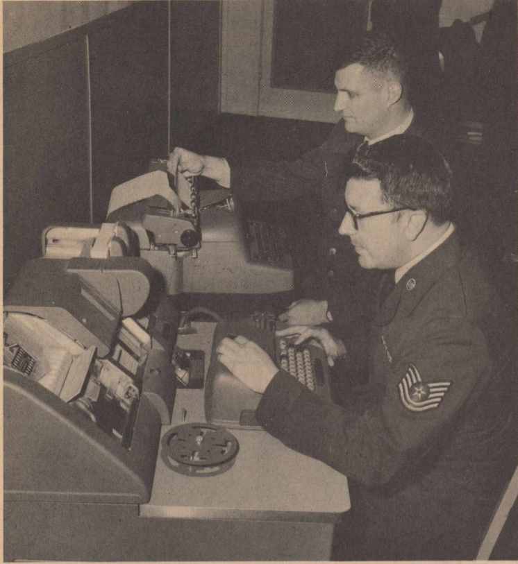
SPECIAL INSTRUCTOR COURSE —NCO's from all ATC Base Personnel Offices are receiving special training in the use of Automatic Data Processing (ADP) equipment at the ATC Instructor School, Randolph AFB. Familiarizing themselves with the operation of a document writer, used to enter new data to punch card records, are TSgt. Karl F. Klein of Stead AFB, Nev., (foreground), and SSgt. Lon Surratt from Reese AFB. Sergeant Surratt was back on his job this week preparing the officer personnel office to assume ADP responsibilities.
