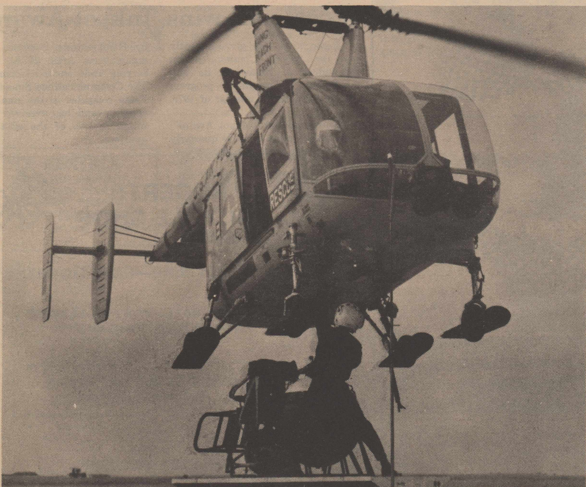
HOOKING UP —Sgt. Wayne A. Cole hooks the fire suppression kit into place as the precision capabilities of the helicopter's pilot keep the aircraft in perfect position for the delicate operation.
