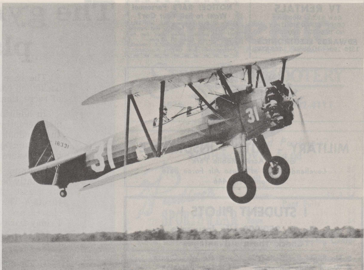
HISTORICAL AIRCRAFT—The Stearman PT-13 was used for primary flight training prior to and during World War II by both the Air Force and Navy. Equipped with a 220-hp. engine, the two-place biplane had a top speed of 135 miles per hour. More than 5,000 copies of the PT-13, in its various configurations, were built. (U. S. Air Force Photo)
