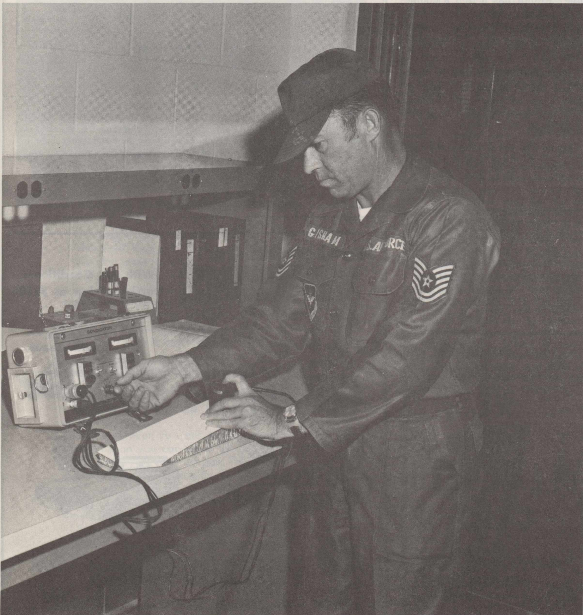
. . . Sergeant Grisham, lab NCOIC, then uses ultrasonic equipment to test for structural damage.
