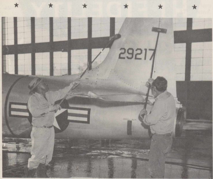
GETTING CLEAN—A T-33 trainer aircraft undergoes a washing, with Albert Lewis, left, and Herminio Lara at work. The pair washes every plane brought in for its 100-hour periodic checkup. About 45 minutes are required to clean each aircraft.
