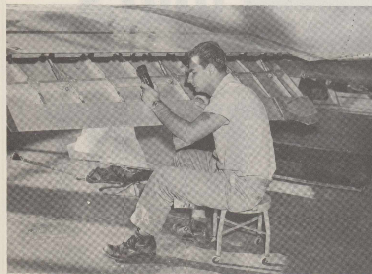
FLAPS—Bill Karon is finishing his part of the 100-hour T-33 check by inspecting the flap assembly of a jet trainer.
