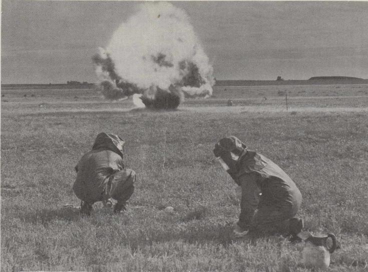
LIQUID OXYGEN mixed with a little oil becomes a dangerous explosive when ignited. Results of such a combination are demonstrated here by two members of an ATC Fire Protection team that visited Reese last week. The explosive qualities of other chemicals and alloys were also ignited as part of a demonstration to show the seriousness of mishandling missile propellants in the event of a fire.
