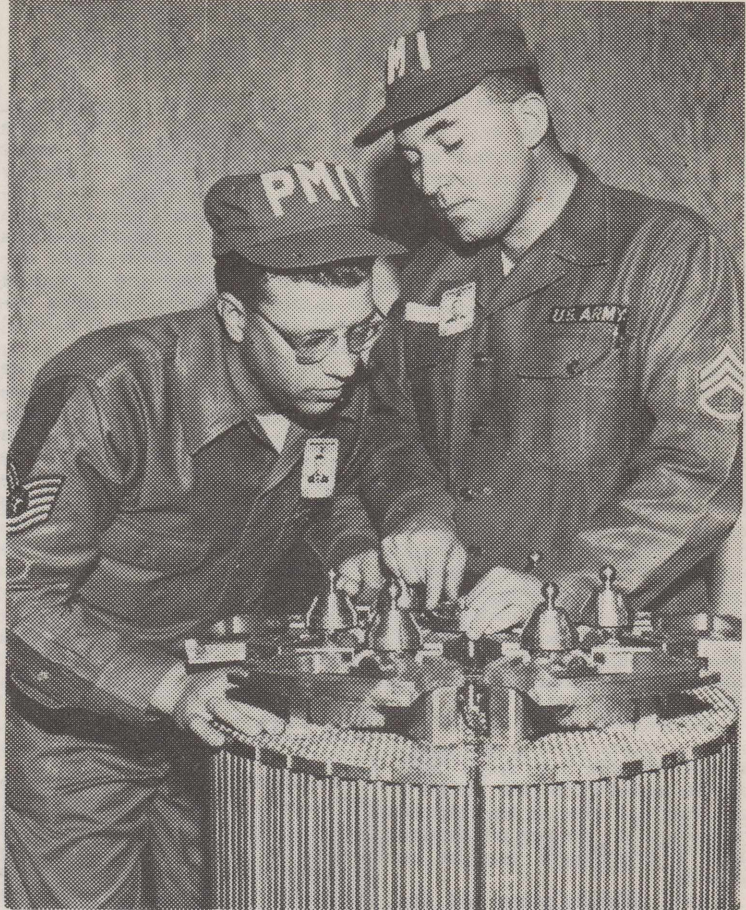
LOOK-SEE —Air Force TSgt. Robert S. Ulrich and Army SSgt. Norman M. Ruskin examine a fuel core for PM-1, the nuclear power plant which will provide heat and electricity for an Air Force radar station near Sundance, Wyo. A single fuel core, lasting two years, will do the job of millions of gallons of diesel oil. Both members of the plant's operating crew, the two men are undergoing training at the Martin Company's nuclear division, where PM-1 is nearing completion.
