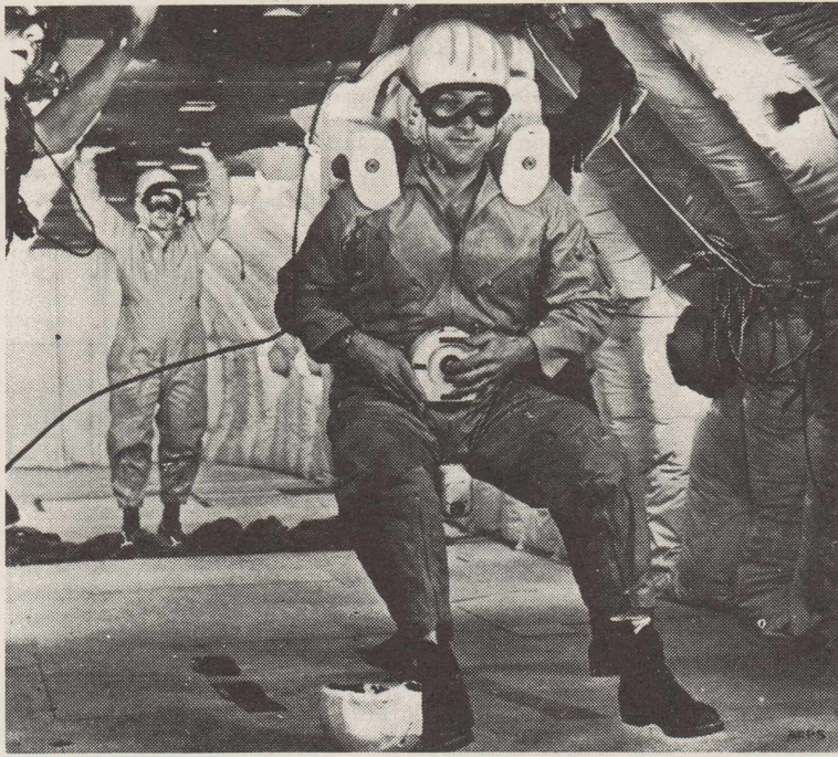
ONE-MAN SPACESHIP —James Griffin demonstrates a compact space pack test model aboard a specially equipped Air Force KC-135 jet transport. Tested in a state of weightlessness aboard the aircraft, the self-manuevering unit is designed to convert an astronaut in a full pressure suit into a one-man space vehicle.
