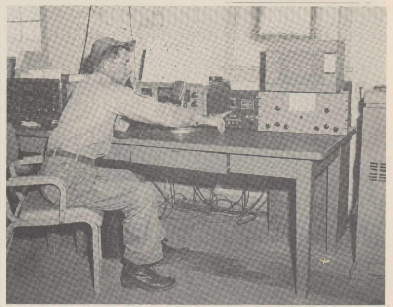
SAVES MONEY — TSgt. Raymond Brady, NCOIC of the MARS station, sets up a patch to complete a call from Reese to Webb AFB. The patch permits use of a telephone instrument at one place for a phone call by radio to another place. Telephone tolls are saved. A call can be placed from here to virtually every military station in the nation. (Photo by Perez)
