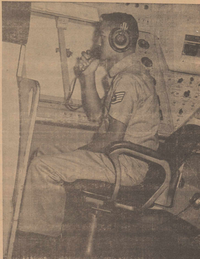
TELLS WHAT —SSgt. Robert Eusebio, instructor, directs a student in simulated flying. Back of him is the panel board on which he can set up any condition of flight, while to his right reactions of the student are recorded.
