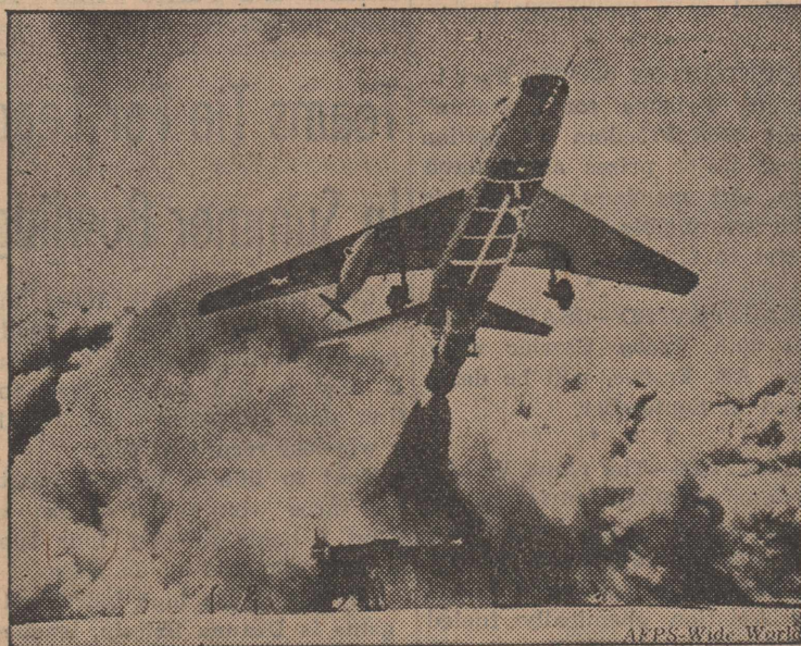
3-2-1-GO — Air Force F-100-D Super Sabre jet leaps from mobile launcher at Edwards AFB, Calif., demonstrating how fighter bombers can become airborne from remote sites without using runways. The F-100-D used the thrust of its own engine plus the kick of a 130,000-pound thrust rocket to get into the air and accelerate to 275 mph in less than four seconds.
