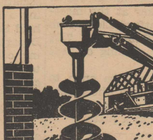
Makes holes for building foundations.
