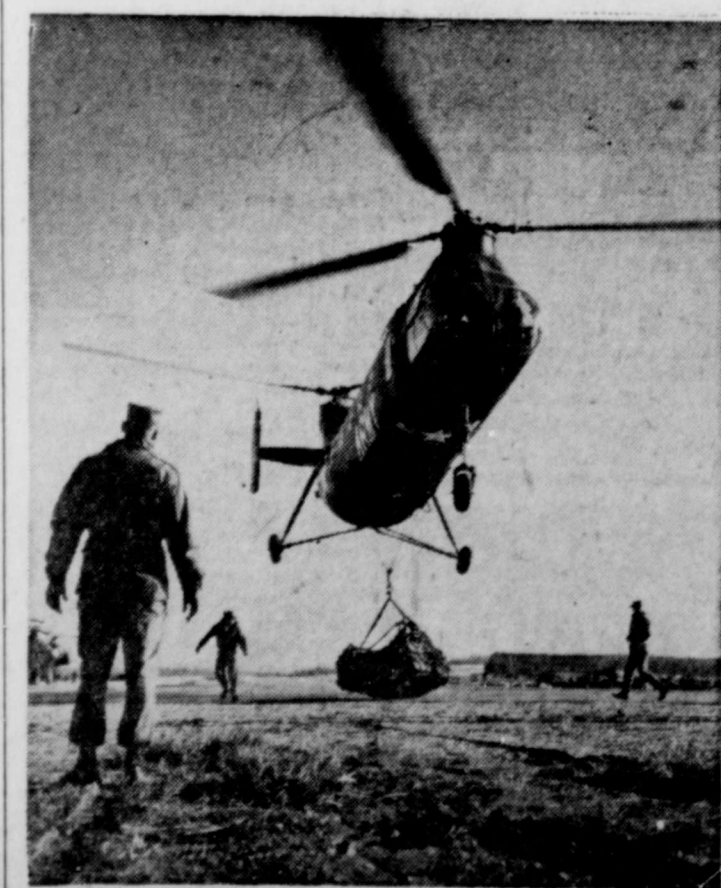
EASY DOES IT—The Army uses the big two-and-a-half ton Piasecki transport helicopter to carry supplies either in or outside the body of the aircraft. Here a cargo-net carrying 2,000 pounds of ammunition is being brought in during training maneuvers at the 59th Transportation Company (Helicopter), Davison Army Airfield, Fort Belvoir, Va.
