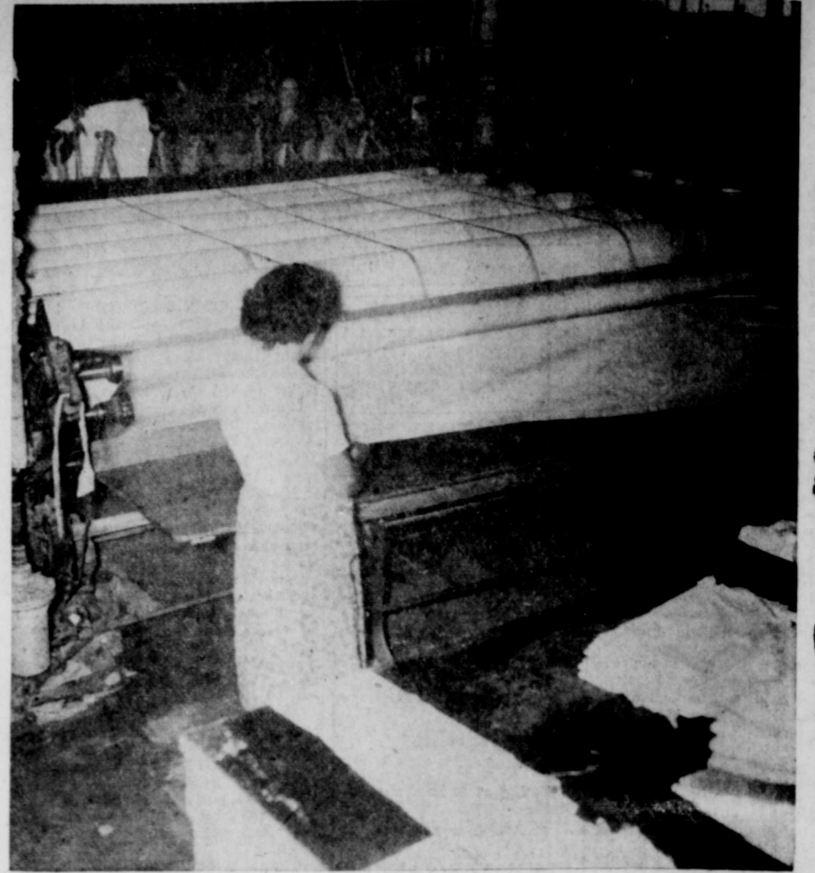
MODERN MACHINES operated by experienced workers insure superior cleaning and ironing of garments and flat goods. For sheets and other large pieces, this dryer-ironer rolls out its work spotless, gleaming and wrinkle-free. In an industry where labor turnover is usually high, nearly every employe has been with the firm several years. (Advocate Photo)
