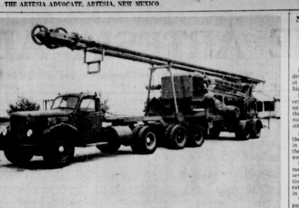
THIS \$30,000 Walker-Near spudder is the third of its type to be brought into North Eddy county, where it will join equipment at the Roland Rich Woolley camp. It is a 5,-000-6,000 foot spudder with a rotary attachment. Fully extended the mast in position is 88 feet high. It is operated by two men, replaces Woolley rig which burned last fall. Similar rigs are owned by Robert E. McKee and Carper Drilling Co. (Advocate Photo)
