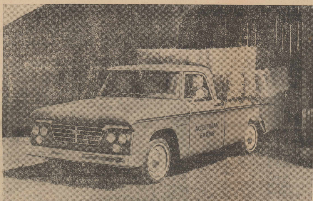
TRUCK STYLE LEADER —At home in the city and on the farm, the 1962 Dodge D-100 Sweptline pick-up features a handsome one-piece stainless steel grille, low hood silhouette and contemporary styling. A highlight of the Sweptline is its 140-horsepower, 225-cubic-inch, Inclined 6-cylinder engine. The truck is available with a 114-inch wheelbase and 6½-foot body or a 122-inch wheelbase and 8-foot body. It has a maximum gross vehicle weight rating of 5,100 pounds.
