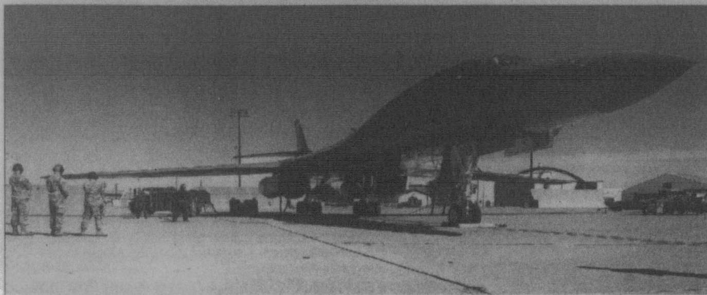
A B-1 Bomber undergoes a hot pit refuel Feb. 22, 2013, at Dyess Air Force Base, Texas. New to the B-1 Bomber, hot pit refueling is a procedure used to rapidly refuel the aircraft while their engines are running, resulting in a speedy refuel. (U.S. Air Force photo by Airman 1st Class Jonathan Stefanko/Released)
