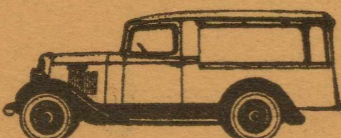
Canopy-top express body on new Half-Ton International. A station-wagon body is also available.
