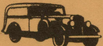
Illustration above shows 6-ft. panel body on 115-in. wheelbase. A 7-ft. body on 125-in. wheelbase also available. Inside height, both bodies, 52 inches.
