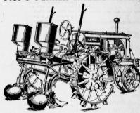
THE No. 22 planting attachment converts the McCormick-Deering No. 3 Farmall Middle Buster into a first-class cotton planter. The planting mechanism is driven from the right-hand rear wheel of the Farmall Tractor.
