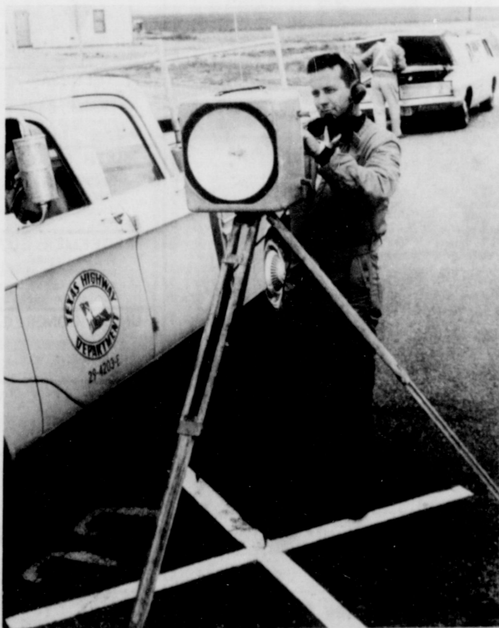
MAKING READING... An engineering technician from the Texas Highway Department's Austin office is shown making a reading in conjunction with the markings which are located along U.S. Highway 60. The series of Xs and squares are all part of the department's system of mapping the road.
