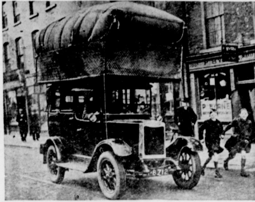
The pinch of war has forced Eire to severely restrict the sale of gasoline. Rationing of "petrol" fails to phase this taxicab driver in Dublin. He has rigged a gas bag to his back's roof and buzzes merrily along, doing 25 miles on one shilling, sixpence (about 30 cents) worth of illuminating gas.
