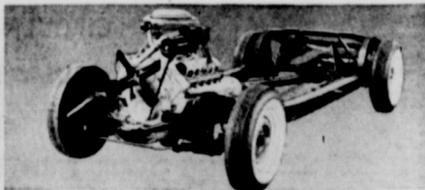
The Dodge frame is built to take it! Massive box-section side rails extend the full length of the frame, are stronger than U-channel or I-beam types used in other cars. Short, rigid brackets anchor the body securely to the frame.
