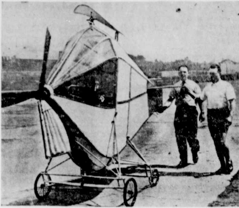
Resembling a winged baby buggy, this peculiar looking contraption is the invention of Paul Fouilleul (right) of Paris. The propeller is powered by pedals. M. Fouilleul has not as yet attempted to take off, but has high hopes that the plane will fly. Ground tests have shown a possible speed of 35 kilometers per hour.
