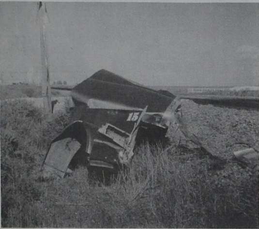
HOOD AND FENDERS from the truck after it was hit by train.
