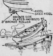
place by means of two bronze side plates. The roller must, of course, turn freely between these plates. A steel or iron roller should not be used, as it soon rusts and! then becomes useless. The roller should' be kept well greased in order to obtain. the best results.
