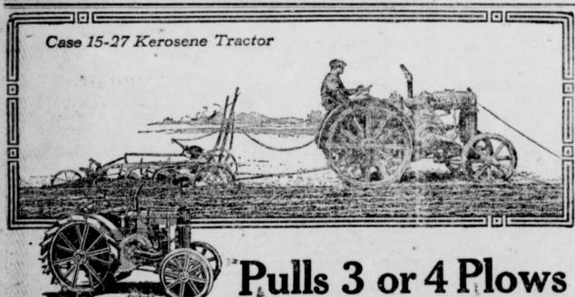
In fields where plowing is difficult—tough or baked soil, stiff grades, etc.—this Case 15-27 Kerosene Tractor will pull 3 plows
