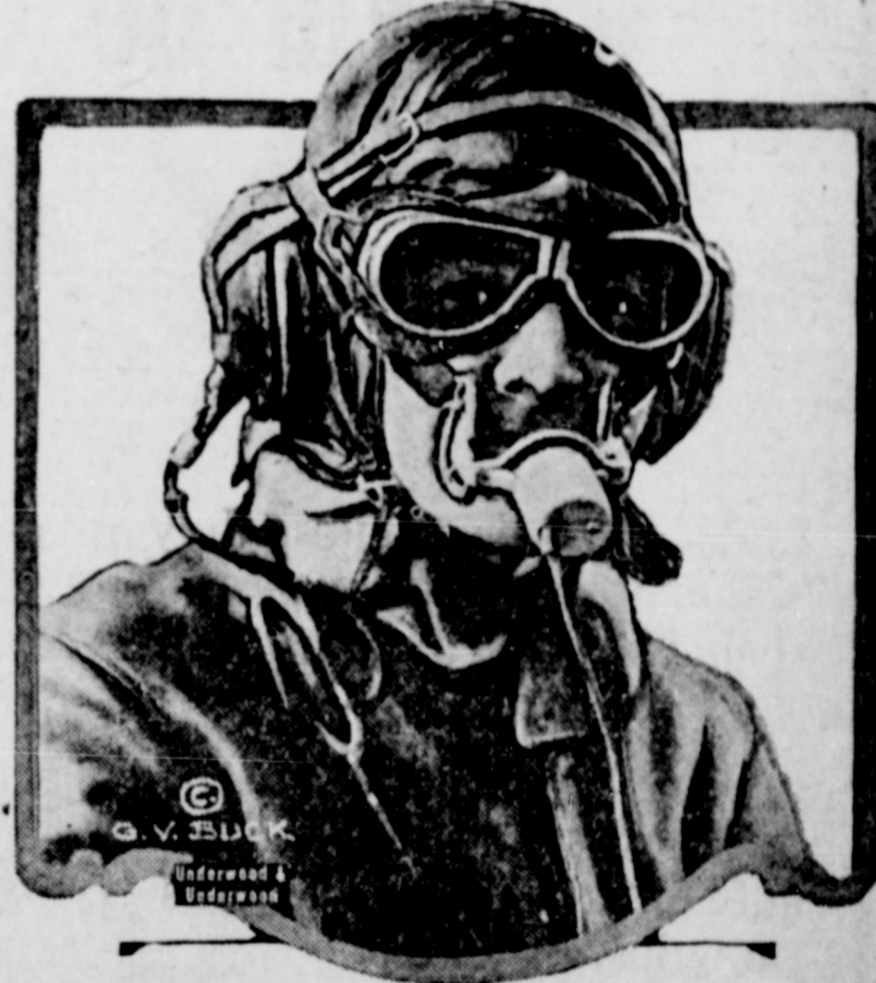
This is the transmitter of the wireless telephone that has been put in successful operation between the land and planes a great distance away. It is worn by the man in the plane.
