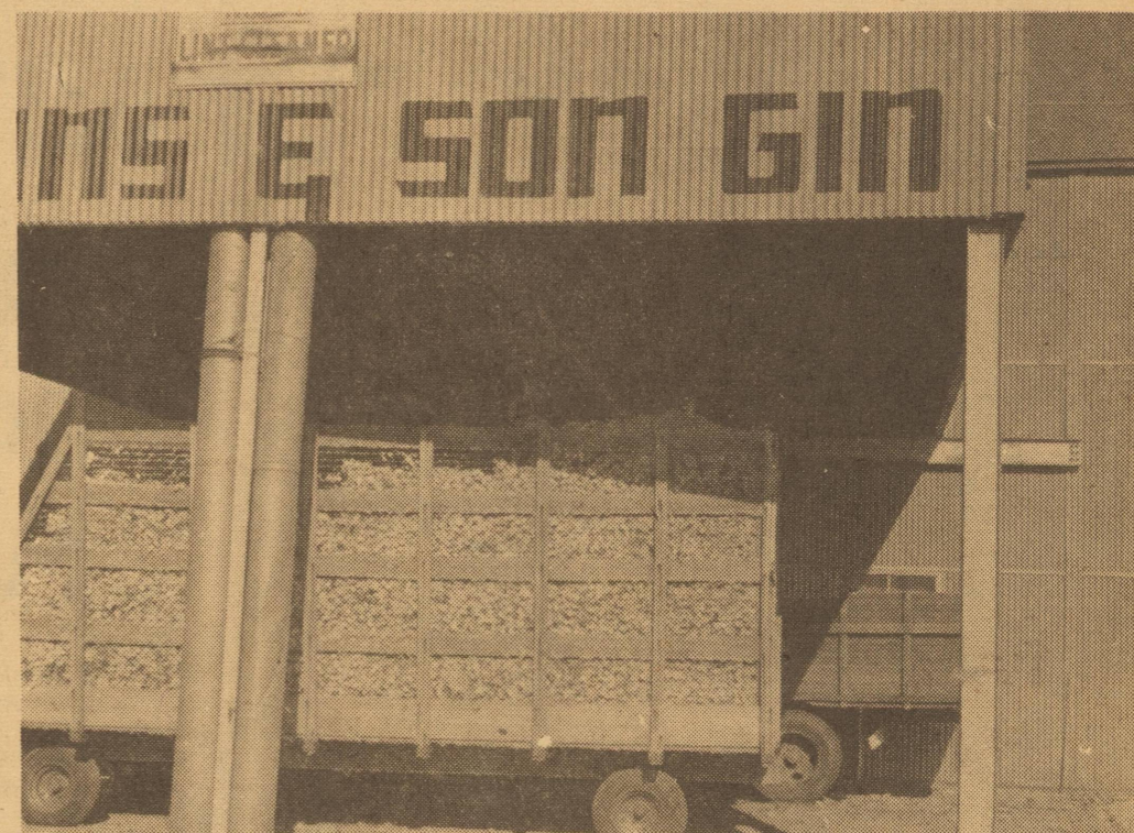
THIS IS THE BUSINESS END of one of the Lazbuddie area gins, which have been running around the clock to get the 1959 crop out. Folks not familiar with cotton production are constantly amazed by the giant suction pipes that pick up bolls for ginning.
