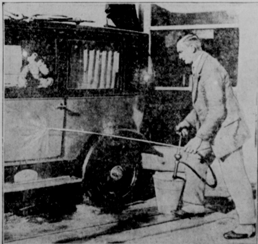
A demonstration of the new portable auto-spray device which has been introduced in Germany. Whether in town or country, the motorist needs only a pail of water, and this hand-spray to clean up his car.
