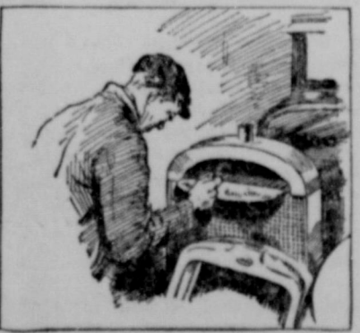
Incision in Radiator, After the Shell is Removed, Gives Access to Obstructing Particles. Remove the radiator shell and with a sharp, strong knife make a curved incision. Then fold out the flap thus formed. Pick out the obstructions with a pointed instrument, push the flap back in place and solder it. Radiators are made of thin sheet brass so this is easier than it looks.—Popular Science Monthly.
