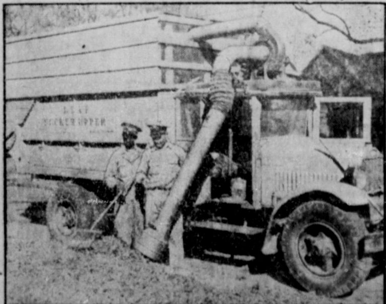
Public works employes at Columbus, Ga., are through with autumn leaf worries, thanks to the ingenuity of one of the city shop mechanics, who designed this "leaf sucker-upper," powered by a three-horsepower gasoline engine. It sucks up the leaves and crushes them for immediate use as a mulch in city parks.
