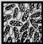
Organic fiber (cellulose)—air is trapped between and IN fibers.
