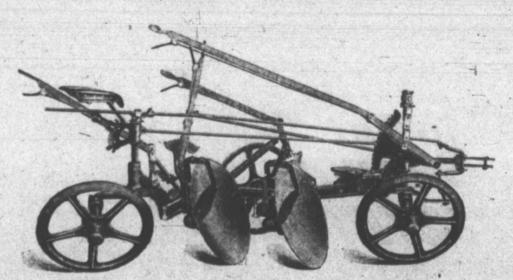
The latest and most up-to-date Disc Plow on the market. Light draft, easy to operate, dust proof, case hardened bearings on both wheels and disc. Will turn to the right as well as to the left. Will plow the hardest of land, both new and old. Goes into the ground by means of principle and not by weight and cuts out a clean furrow.
