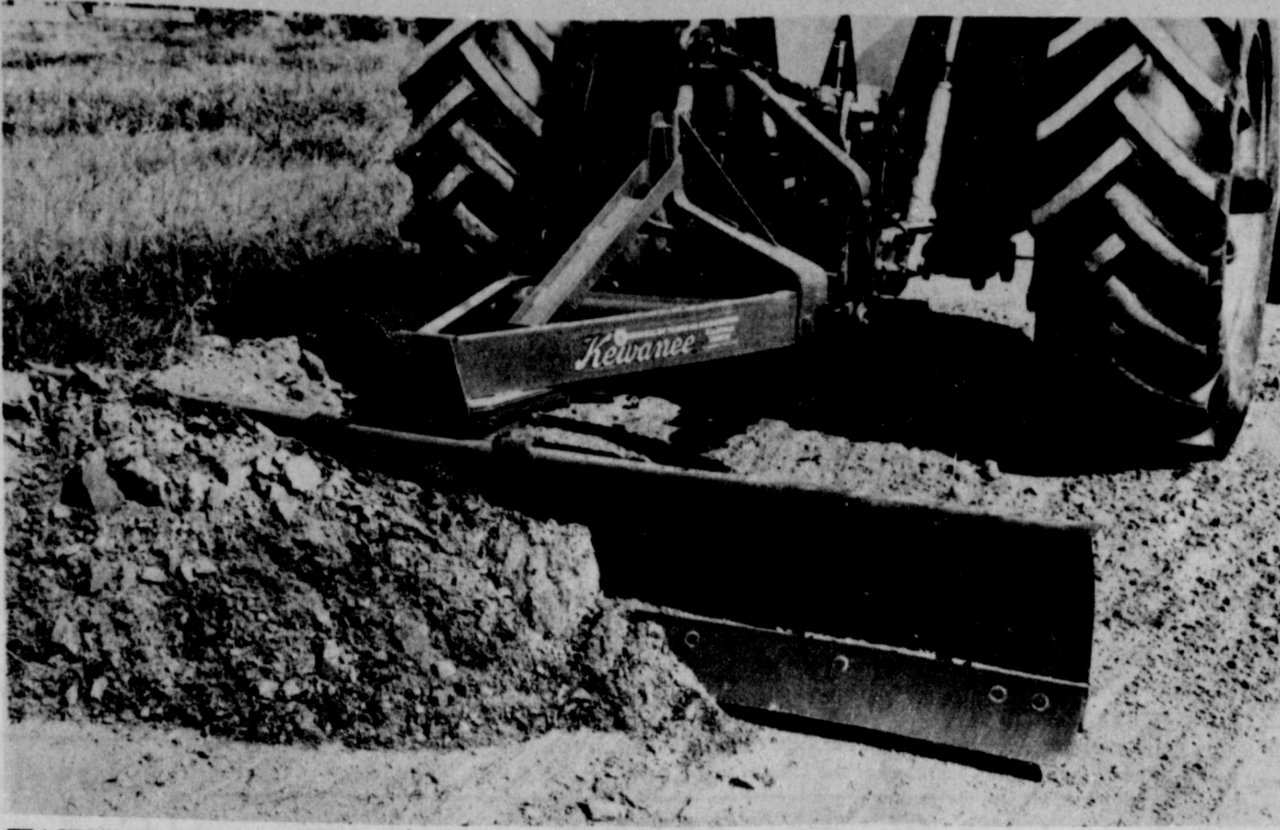
TRACTOR BLADES are designed to push or pull things -- not hit them, according to Howard Hadler, Division Engineer with Kewanee Machinery Division. He advises farmers to take time, moving big loads with two or three passes rather than taking the whole load at once.
