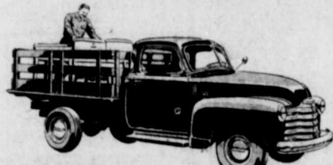
MEDIUM-DUTY DE LUXE STAK* Model 3609—125 1/2-inch wheelbase, Maximum G.V.W. 5,800 lb. Other models available up to 161-inch wheelbase and 16,000 lb. G.V.W.
