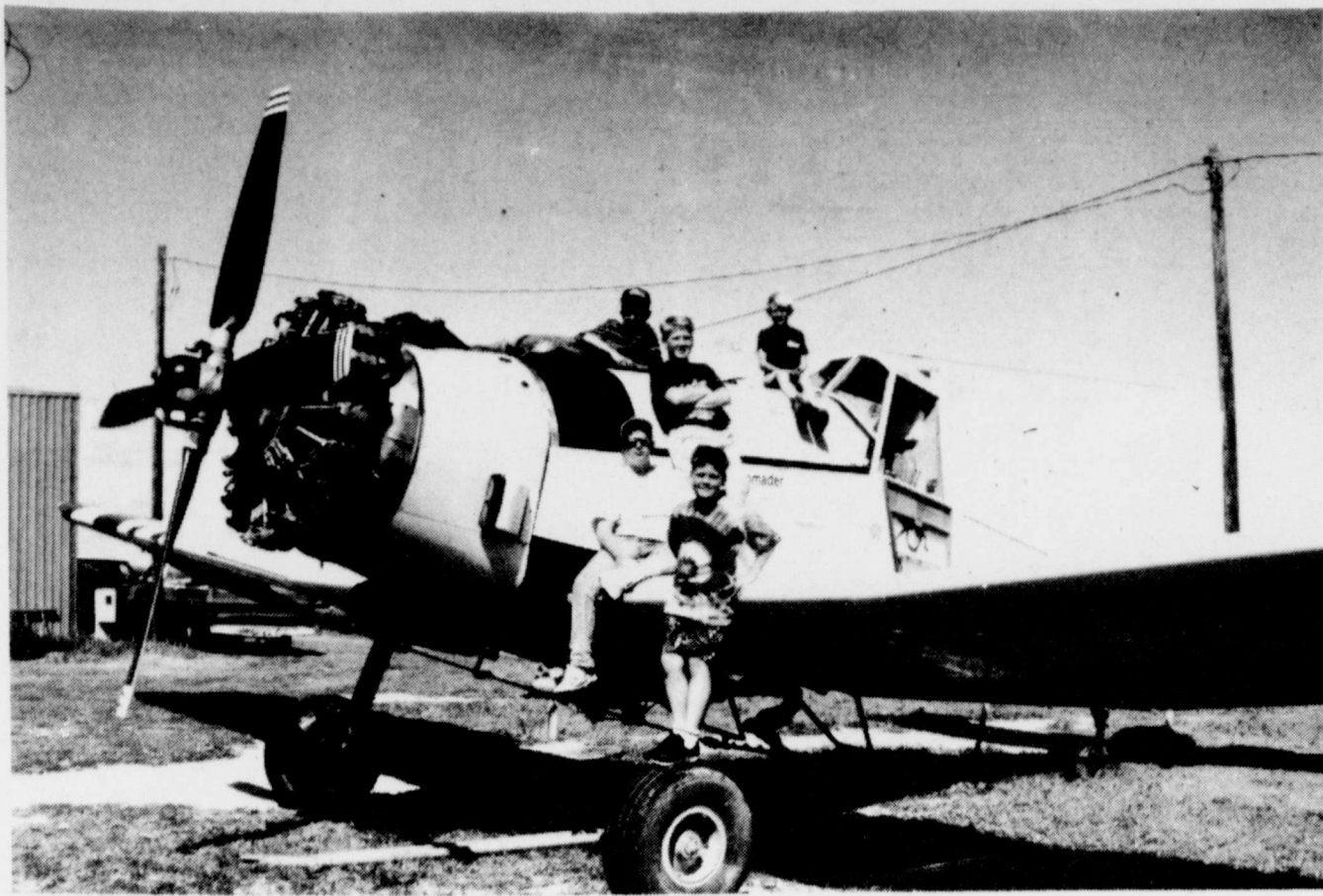
FUTURE PILOTS? — Enjoying some "hands on" experience during "Fly Days" were these Winters youngsters: (top) Kris and Kevin Ballard, (center) Blake Smith and (bottom) Michael Prewit and Ryan Smith. The plane, owned and operated by Steve Ballard of Ballard's Crop Dusting Service, is an M18 Dromader spray plane made in Poland. Having a 58' wing, 1,000 hp engine and the ability to carry 700 gallons of liquid, it is the largest production spray plane in the world and the only one in Texas.
