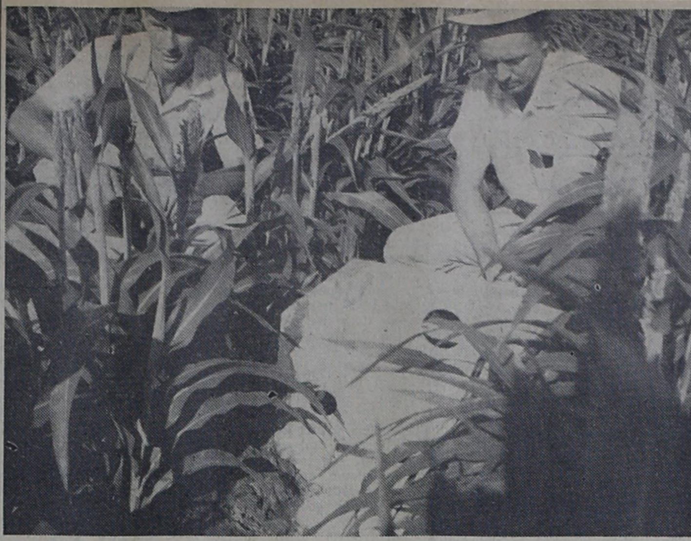
IRRIGATION WATER APPLICATION STUDIES are made with interesting devices. This one is placed in the row in the field, and water flows through the orifices, indicating the rate. Holding the equipment is Bob Crozier. Beside him is Robert Zetzsche. Both are SCS technicians.
