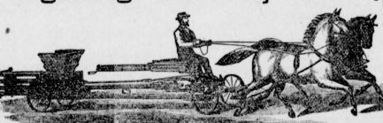
Rapid, Powerful and Durable. Being Very Light, can be drawn by one pair of horses. Set up for use in five minutes. Bales Damp Hay just as well as dry. Tying and Threading from same side of Press. Simple in Construction. Little or No Expense for Repairs.
