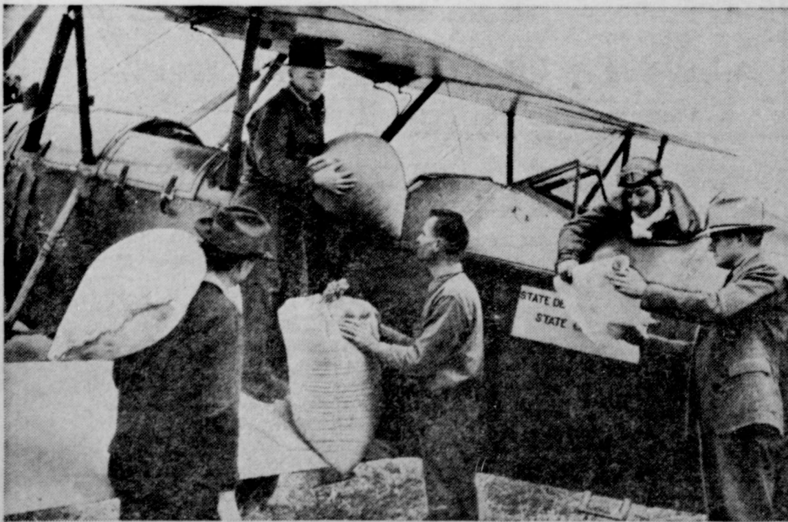
One of the former mail planes used by the government which is now being used to scatter seed over burned-over forest land. The compartments once used for mail have been rebuilt as seed bins with trap doors in the bottoms which can be released by the pilot. The planes carry about 300 pounds of seed.
