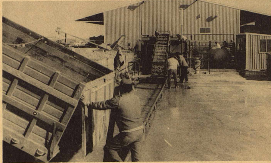
A NEW carrot-processing plant is in operation in Uvalde. The vegetables come into this plant (lower picture), are emptied into a long flume filled with water, are lifted by conveyor to washing drums where they are also chilled with ice water, then go to sizing machines. Discards go one way and the other carrots are sent to grading conveyors where they are hand examined (top picture) for size and texture, then are weighed and packaged. The plant employs about 100.
