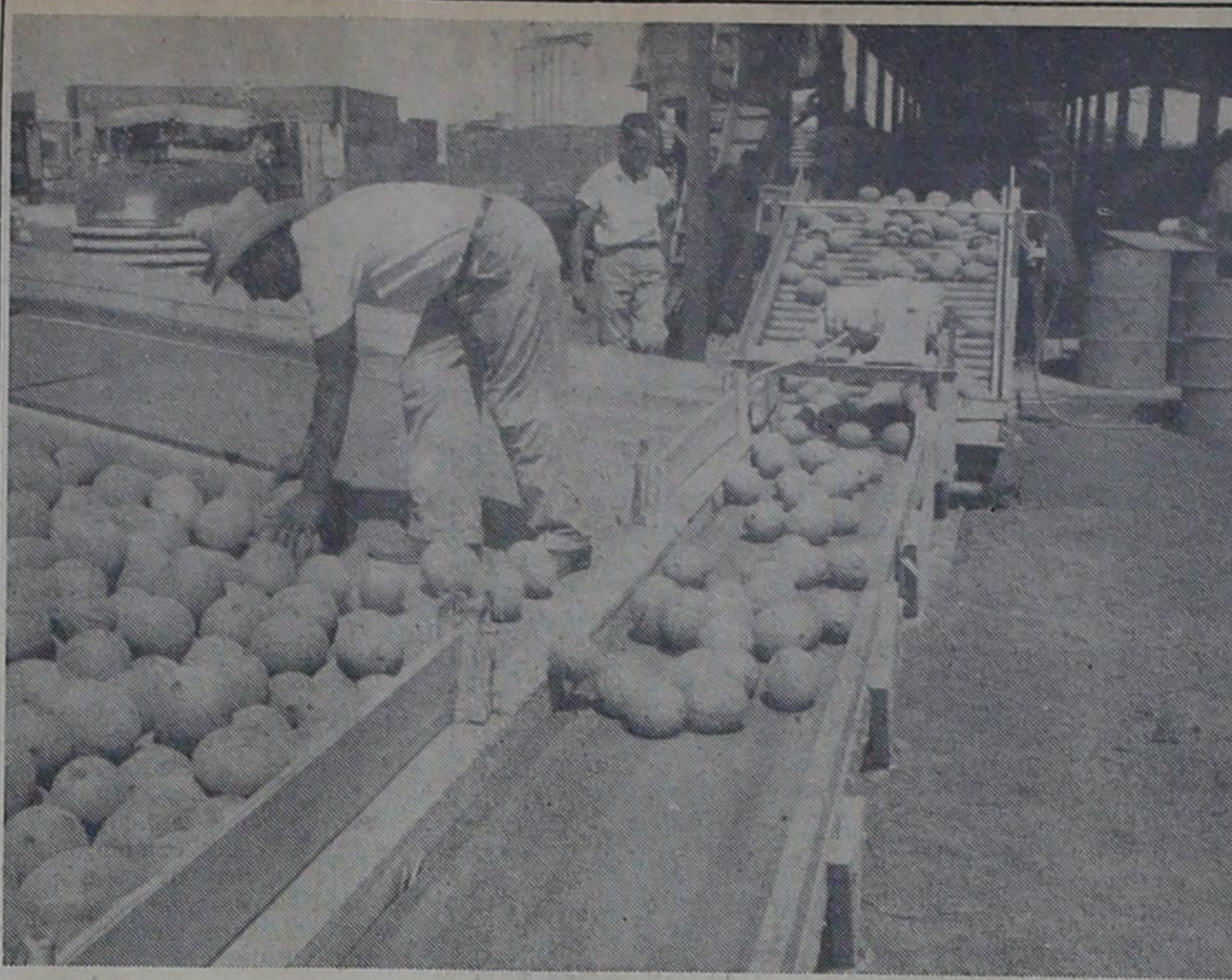
ROLLIN' 'EM IN to the Gateway Produce Company's processing operation is this shed hand who lifts small wooden gates and starts the cantaloupes gently tumbling down to meet a conveyer belt, where they are lifted into the shed. Once inside they are graded and packed by hand.
