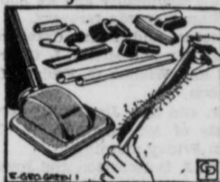
Vacuum cleaner brushes and cylinders will not perform properly if clogged with threads, hair or lint. Remove and clean them often.
