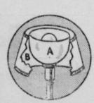
FOR THE STUDY TABLE, an I. E. S. Better Sight Lamp, equipped with 100-watt bulb, gives several times as much light as ordinary lamps using the same amount of current. Glass diffusing bowl (A) sifts out harmful glare. White shade lining (B) reflects maximum light on work. Table models, \$3.95. Three-light floor models, with 100-200-300 watt bulb, \$7.95 up.
