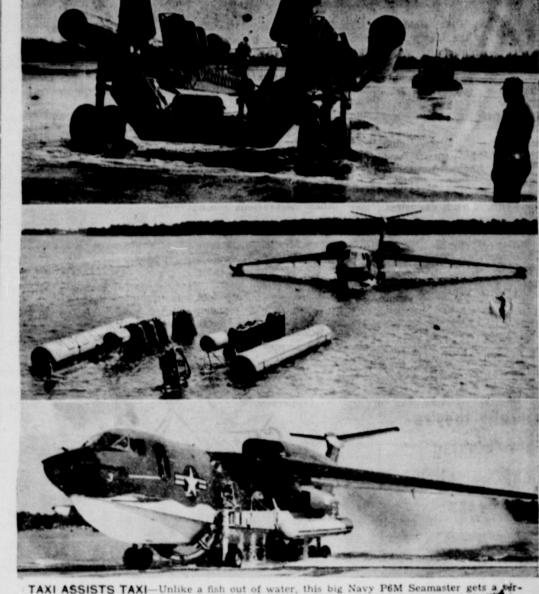
TAXI ASSISTS TAXI—Unlike a fish out of water, this big Navy P6M Seamaster gets a serrestial taxi ride from a newly developed beaching vehicle at the Martin Company's Ball fore seadrome. Top photo shows the device ushered into the water. The Seamaster, center photo, heads for the floating taxi whose hydraulic pads will grasp the plane's hull. On land, bottom photo, the P6M, nestled in the beaching vehicle's cradle, taxies under its own power.
